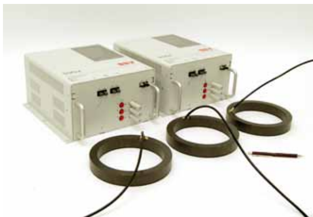
Figure 10.3 Example of FOCS measuring system for AC
