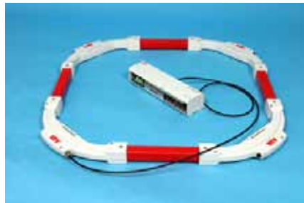
Figure 10.4 Example of FOCS measuring system for DC
