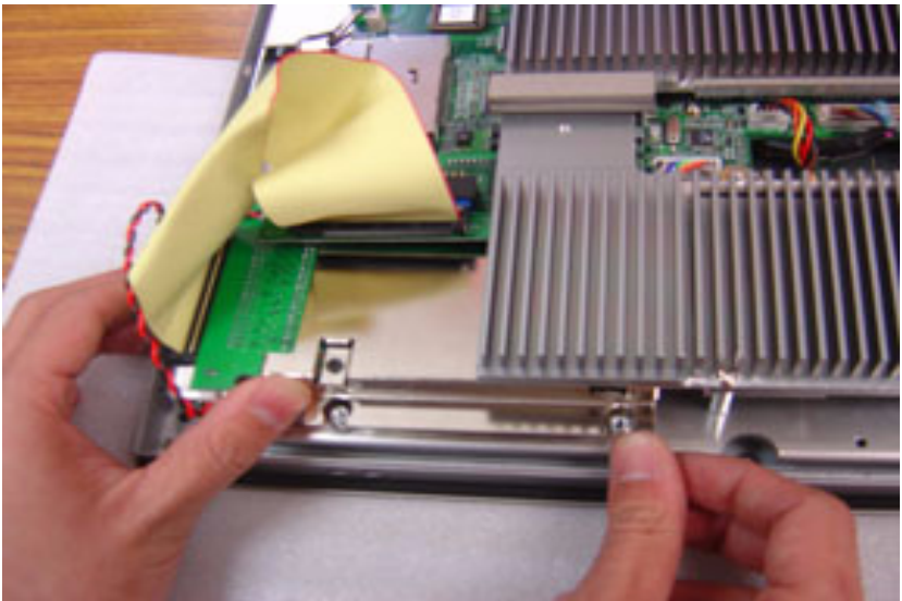
Figure E.12: Completed HDD Installation
