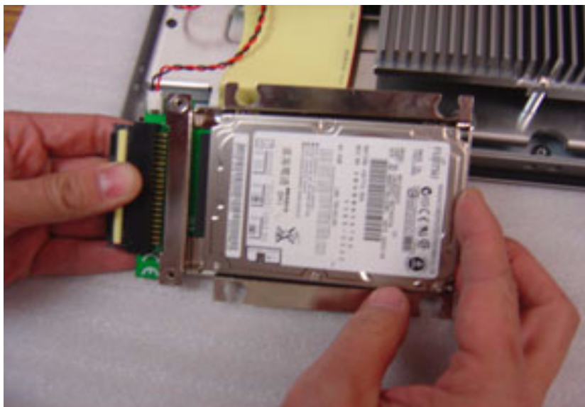
Figure E.6: Installing the HDDr
