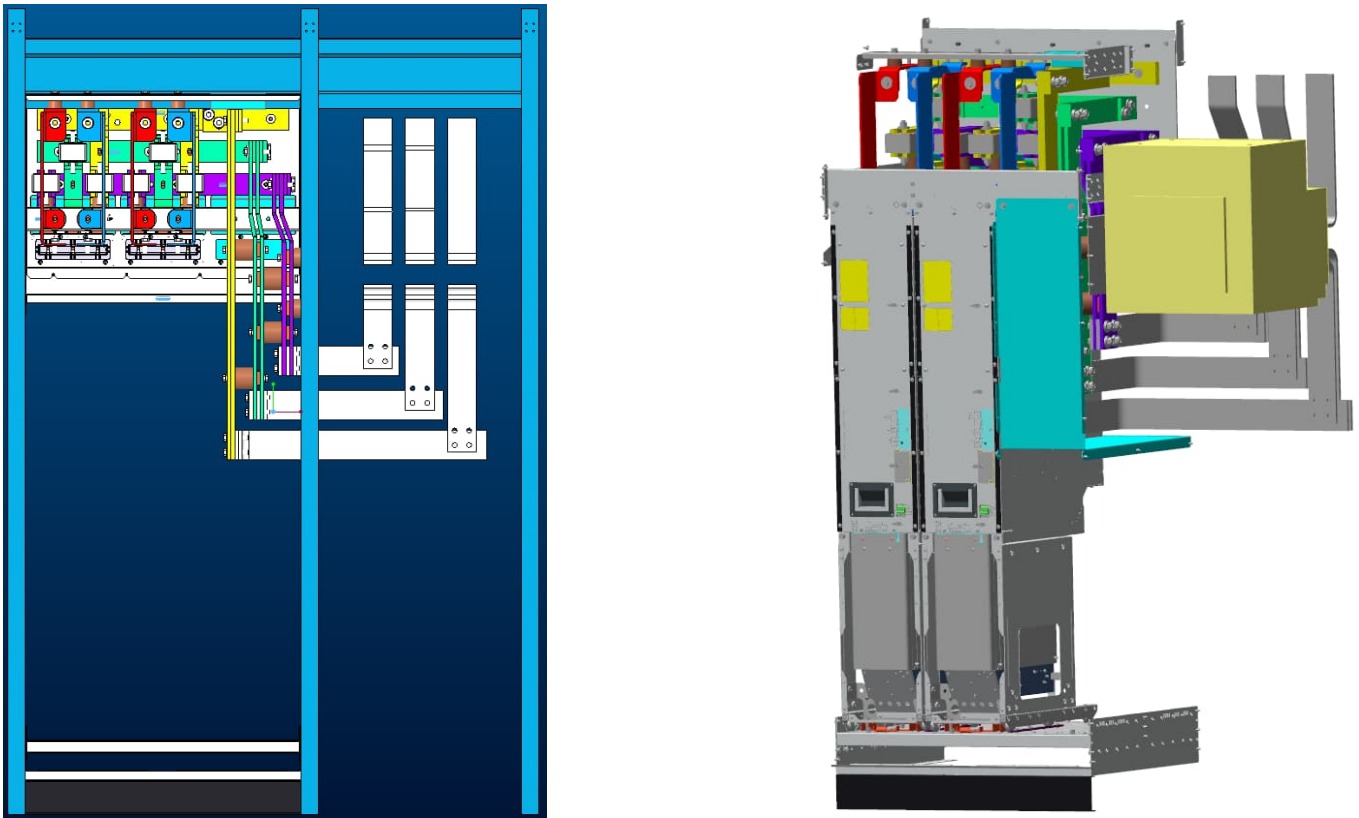
Pic 53. ACS880R-307SS (2XD8T Right) retrofit (kit) solution for Diode supply section of Star/ACV700
